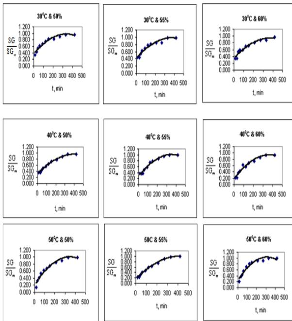
Figure 2. Variation of  $\frac{SG}{SG_{\infty}}$  with time at different combinations of temperatures and sugar concentrations.
