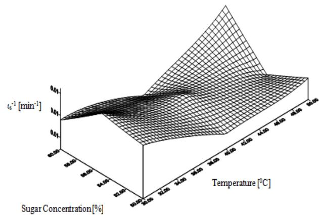
Figure 4. Variation of solute uptake rate constant ( $\alpha_s^{-1}$ ) with temperature and concentration of sugar solution
