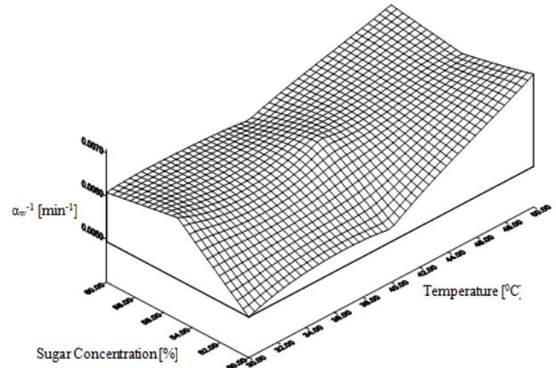
Figure 3. Variation of water loss rate constant ( $\alpha_w^{-1}$ ) with temperature and concentration of sugar solution
