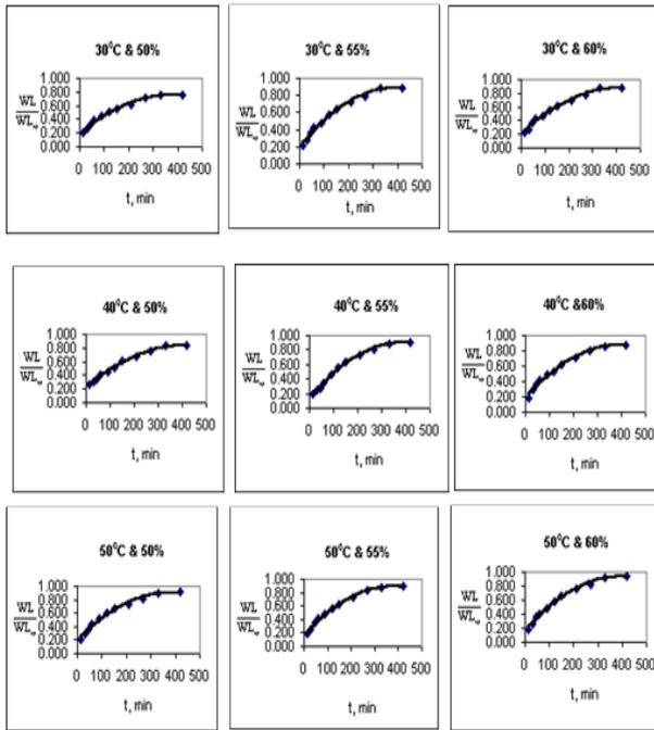
Figure 1. Variation of  $\frac{WL}{WL_{\infty}}$  with time at different combinations of temperature and sugar concentrations.
